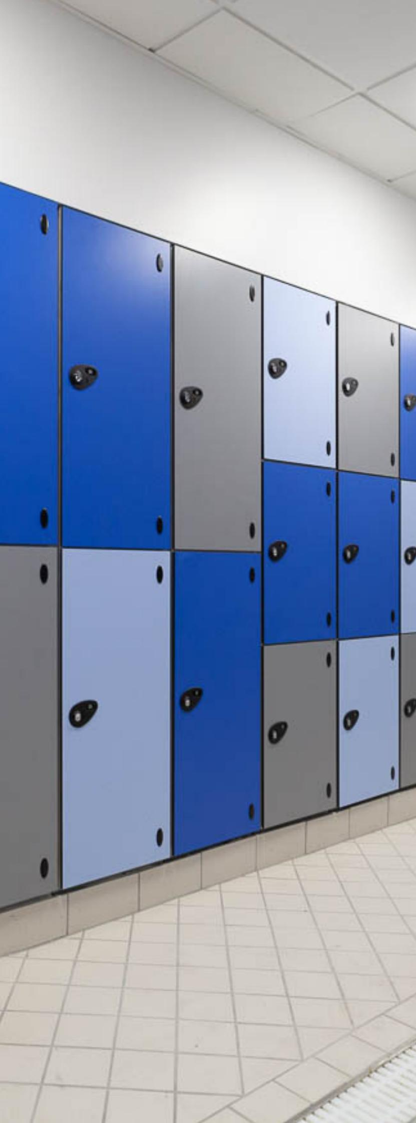
Our Leisure Lockers are specifically designed for areas subjected to chlorinated and high moisture and humidity. Manufactured on-site from aluminium with radised internal corners and feature solid grade high-pressure laminate doors. They are ideal for use in areas of high moisture and humidity as its solid core construction means there is no risk of peeling, cracking or delamination.
