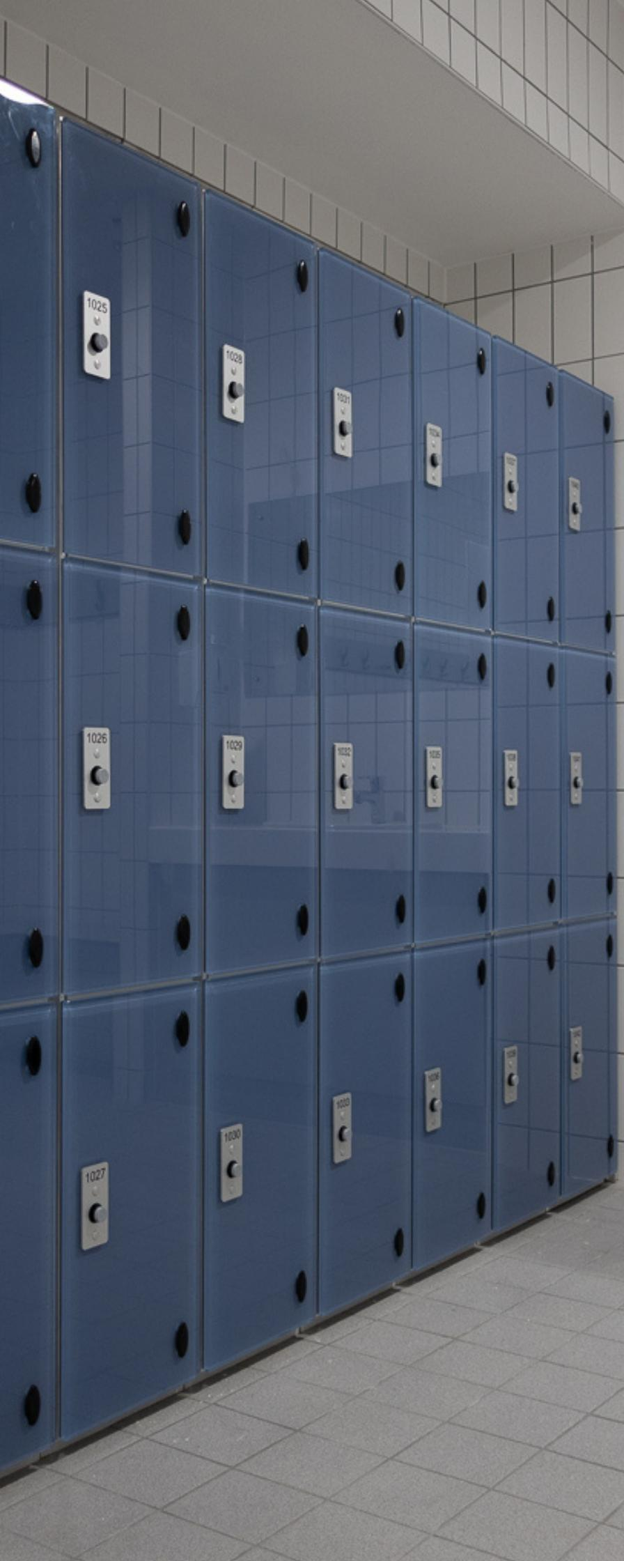
Glass locker bodies are manufactured from aluminium and locker doors are from PAR 10mm toughened coloured glass with a roller coat paint finish inside the locker door.
